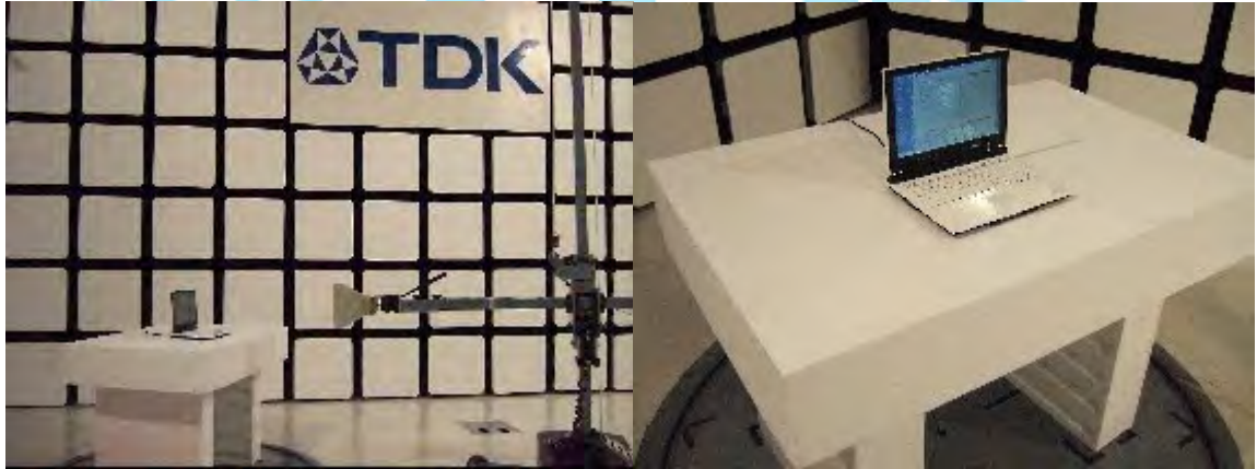
Test Configuration 1. 960 MHz to 40 GHz
