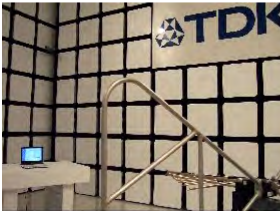
Test Configuration 2. 30 MHz to 960 MHz
