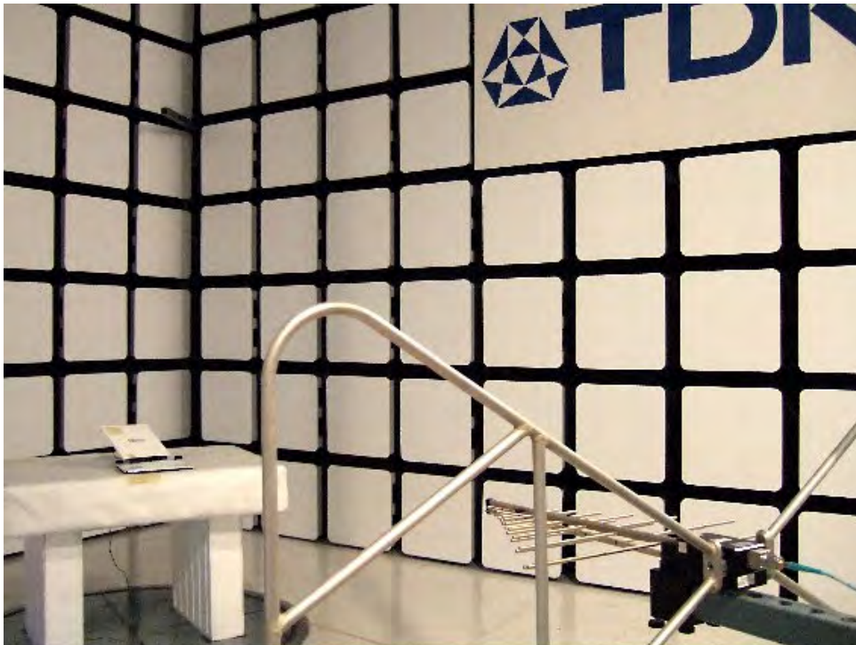
Test Configuration 3: 30 MHz to 960 MHz
