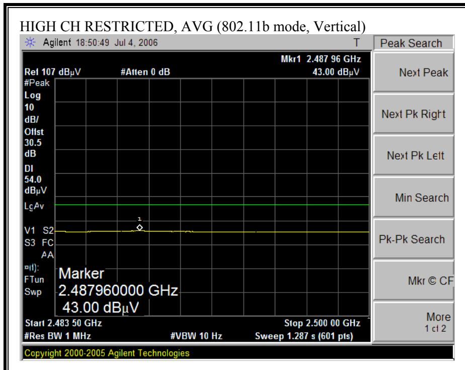
**PORTABLE CONFIGURATION HARMONICS AND SPURIOUS EMISSIONS (b MODE)**
