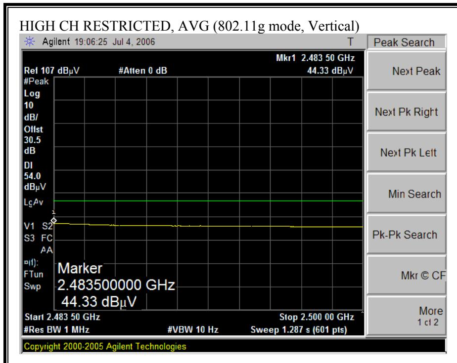
**POTABLE CONFIGURATION HARMONICS AND SPURIOUS EMISSIONS (g MODE)**
