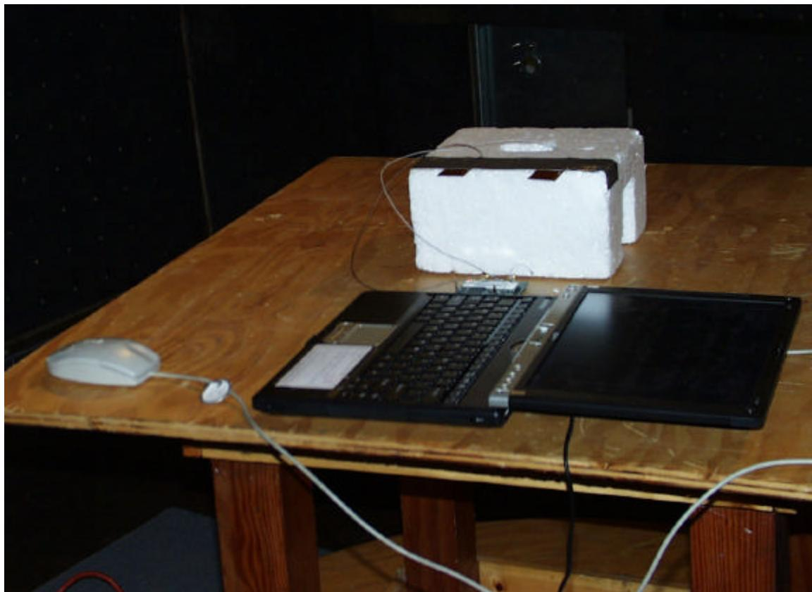
**RADIATED RF MEASUREMENT SETUP: ANTENNA IN Y-AXIS ORIENTATION**
