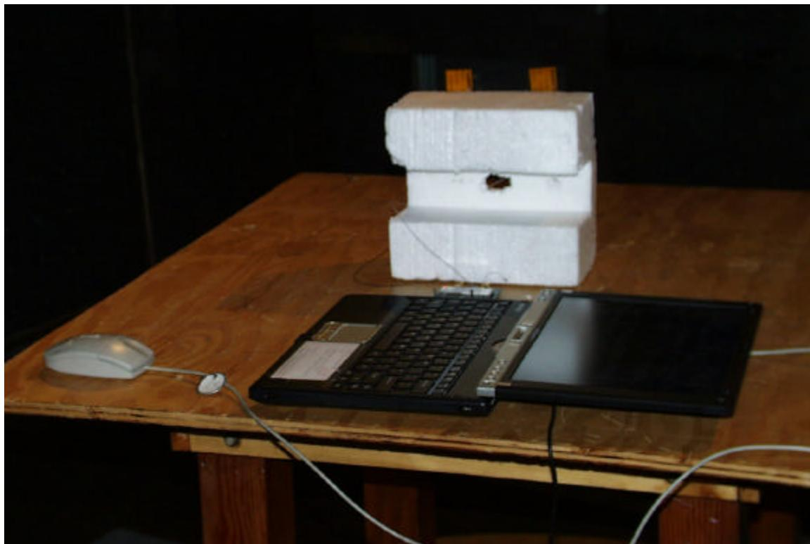
**RADIATED RF MEASUREMENT SETUP: ANTENNA IN Z-AXIS ORIENTATION**
