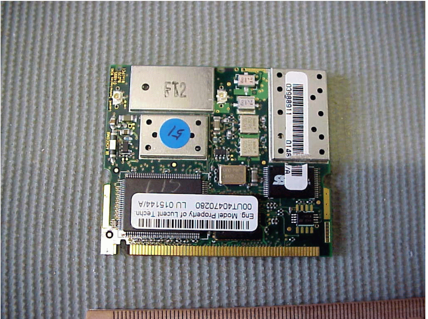
Mini PCI Wireless LAN board - upper side with shield
