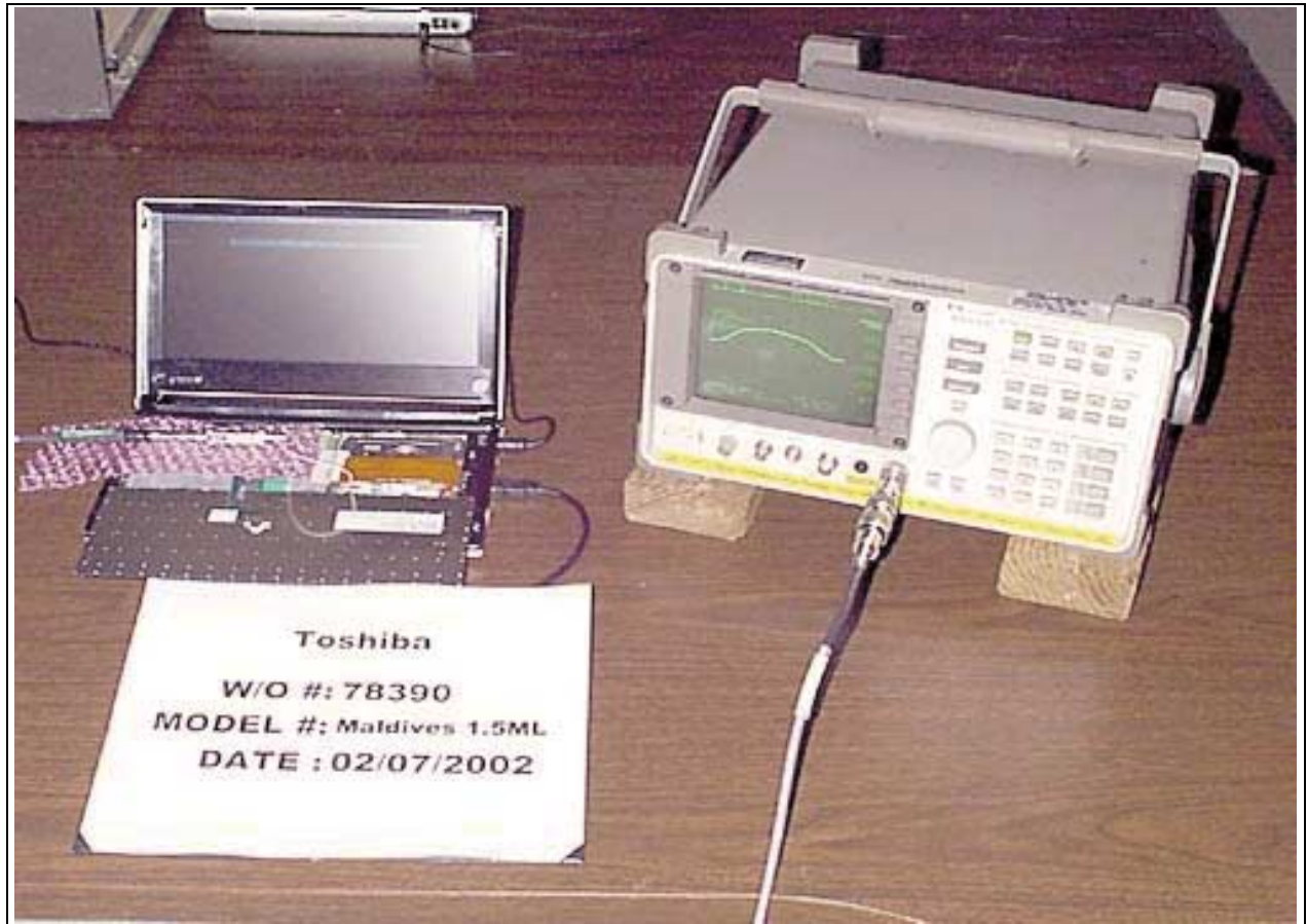
Antenna Conducted Emissions - Front View
