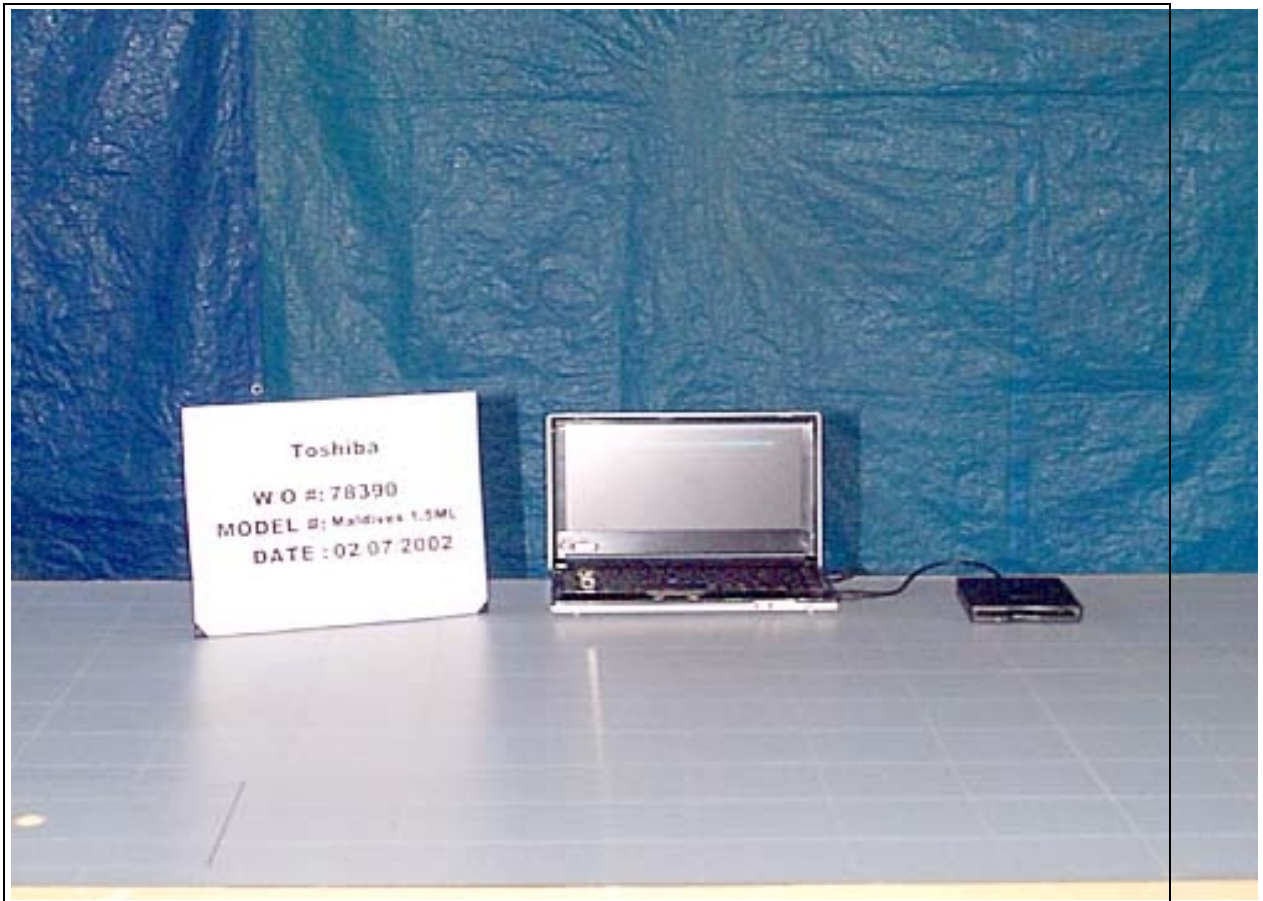
Radiated Emissions - Front View
