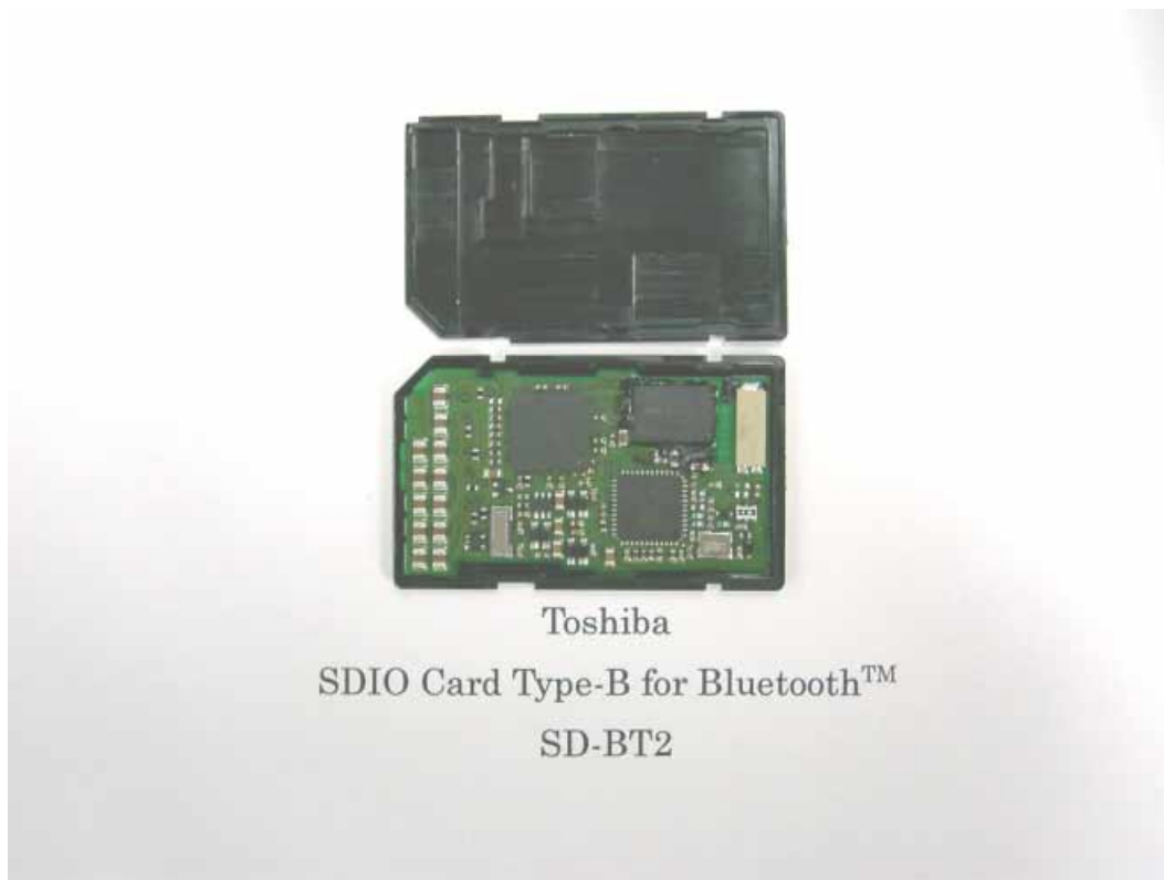
Photo-3: Top Cover Removed
