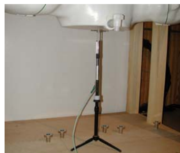
Figure 12.1 Dipole Validation Test Setup
