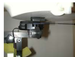
Figure 14.17 Body SAR Test Setup -- w/ Holster --
