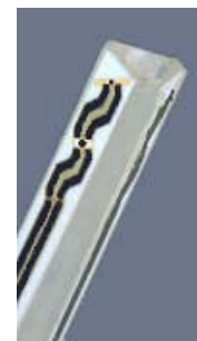
Figure 3.2 Probe Thick-Film Technique
