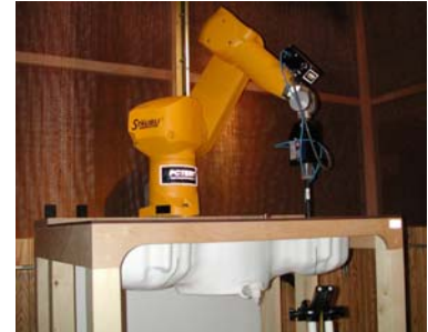
Figure 6.1 DASY3 Test System
