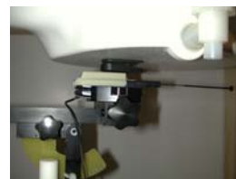
Figure 14.15 Body SAR Test Setup -- w/ Belt Clip --
