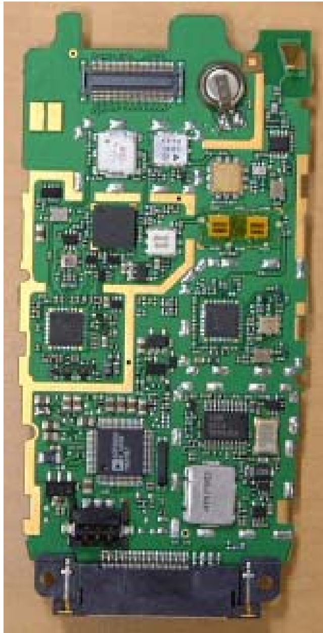
Handheld Portable MAIN Board (Back side , With shield cover removed) VCTCXO : VC-TCXO-208C3-19.2MHz
