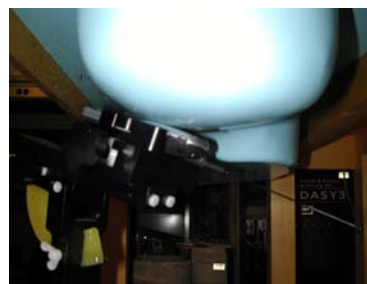
Figure 21. Left Head SAR Test Setup -- Cheek / Touch Position --
