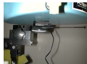
Figure 27. Body SAR Test Setup -- with BeltClip --
