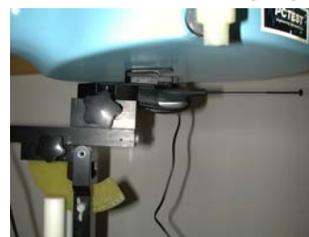
Figure 26. Body SAR Test Setup -- with Holster --
