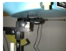
Figure 30. Body SAR Test Setup -- with Holster --
