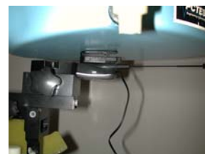
Figure 29. Body SAR Test Setup -- with BeltClip --
