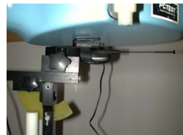
Figure 28. Body SAR Test Setup -- with Holster --
