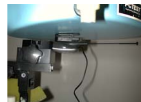
Figure 25. Body SAR Test Setup -- with BeltClip --
