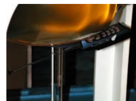
Fig. 15 Head SAR Test Setup
