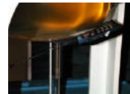
Fig. 17 Head SAR Test Setup
