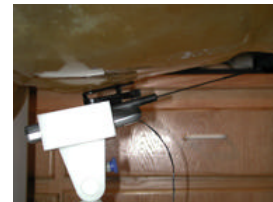
Fig. D Head SAR Test Setup
