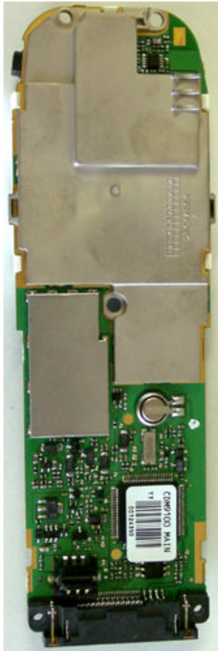
Handheld Portable MAIN Board (Back side , With shield cover)
