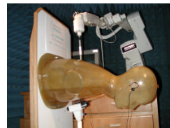
Fig. 1 SAR Test Setup
