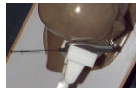
Fig. 14 Head SAR Test Setup
