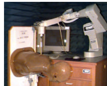
Fig. 1 SAR Test Setup
