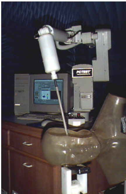
Figure 5. Photograph of the Probe and the Phantom
