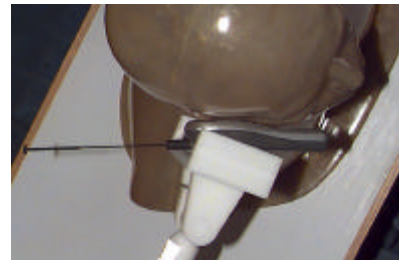
Figure 15. Head SAR Test Setup
