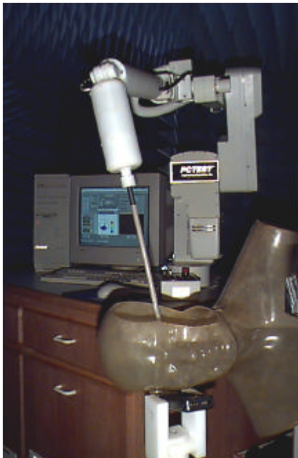
Figure 5. Photograph of the Probe and the Phantom
