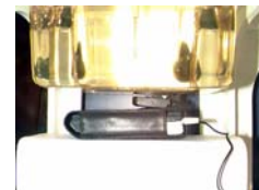
Figure 14.3 Body SAR Test Setup -- w/ Holster & Belt Clip --
