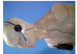
Figure 13. Shirt Pocket Configuration
