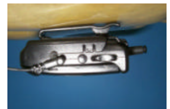
Figure 14. Body Holster Configuration
