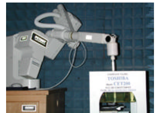
Fig. 1 SAR Test Setup
