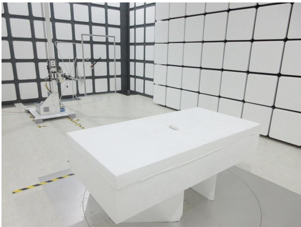
**Test Mode: Mode 1****Description: Radiated Emission Test Setup for above 1GHz**
