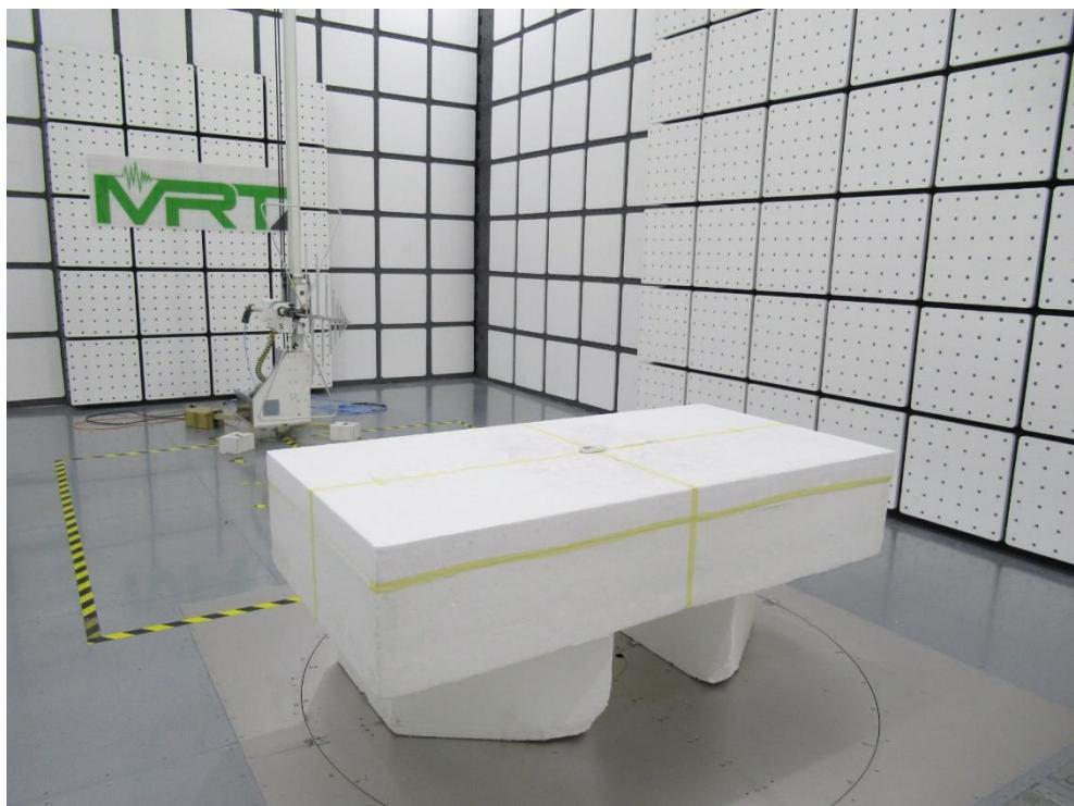
**Description: Radiated Emission Test Setup for above 1GHz**
