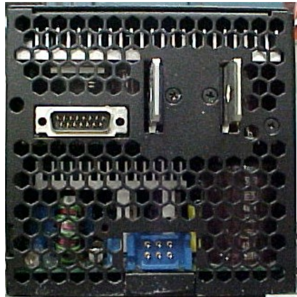
Figure 14: Rectifier plug-in module rear panel.
