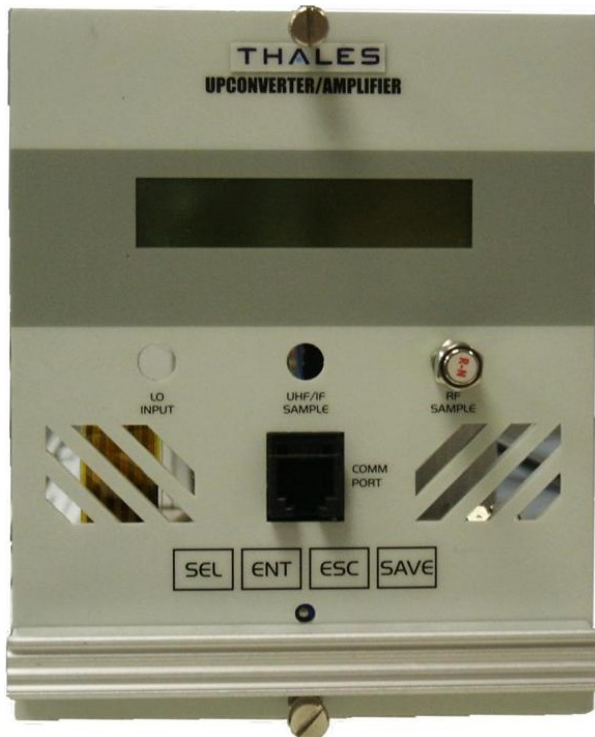
Figure 19: Upconverter module front panel.
