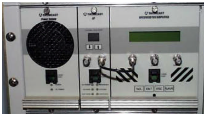
Figure 1: Cabling the LO signal.
