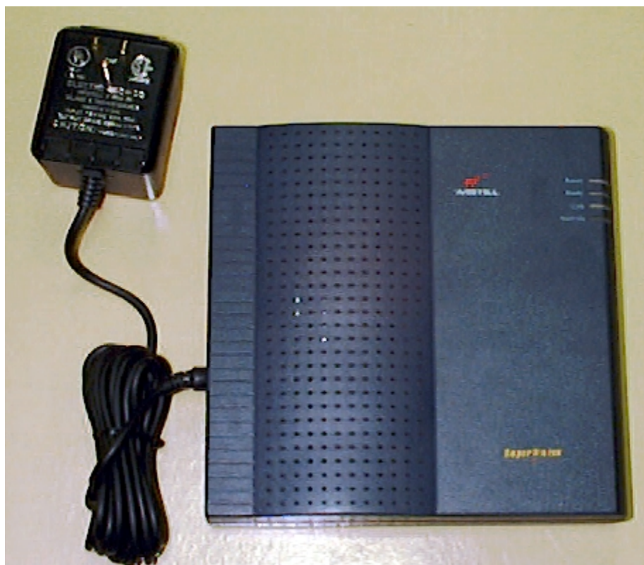
Top of EUT showing AC-AC power supply
