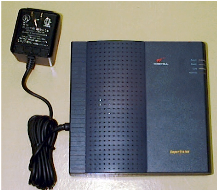
Top of EUT showing AC-AC power supply
