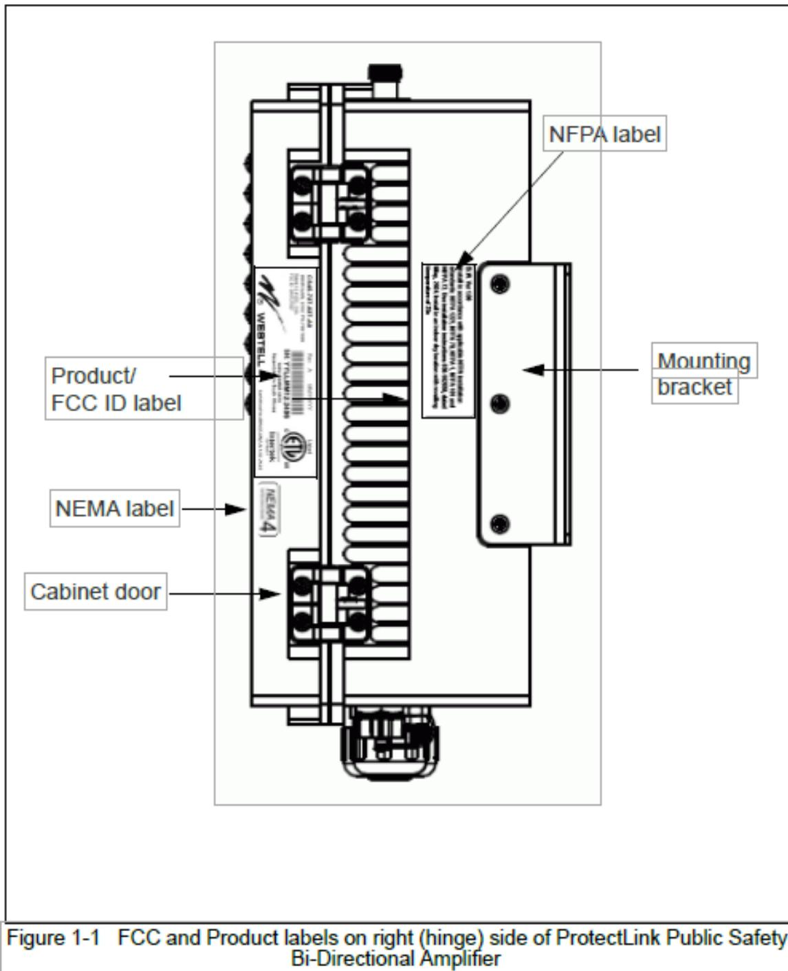
Figure 1-1 FCC and Product labels on right (hinge) side of ProtectLink Public Safety Bi-Directional Amplifier
