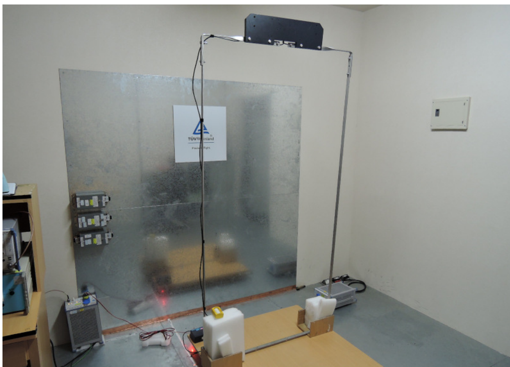
Photograph 7: Set-up for Mains Conducted testing Front
