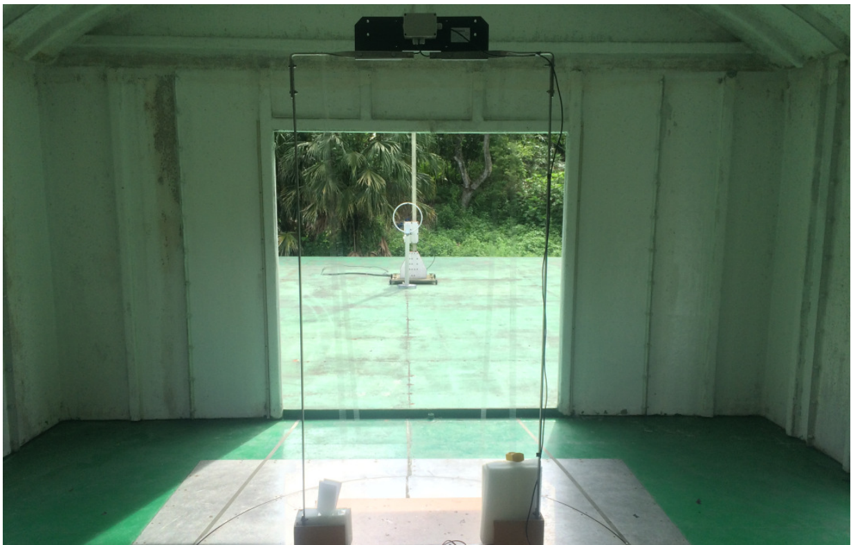
Photograph 5: Set-up for Fundamental Emissions (Single Loop Walk Through antenna)
