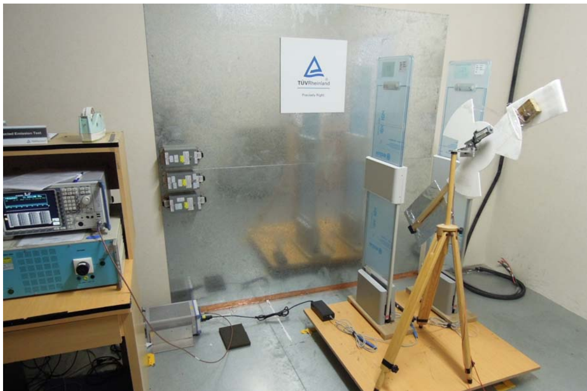
Photograph 5: Set-up for for Mains Conducted testing Front
