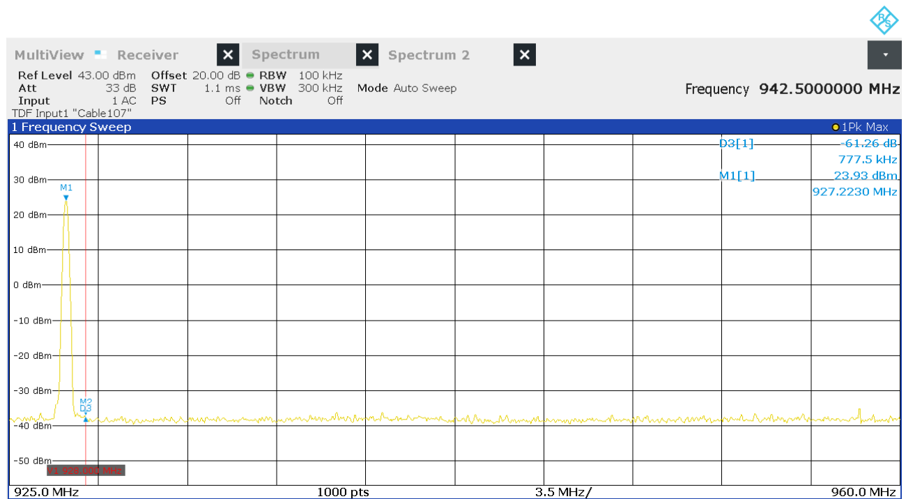
Figure 23: Chart of upper band-edge measurement in non-hopping mode on highest channel
