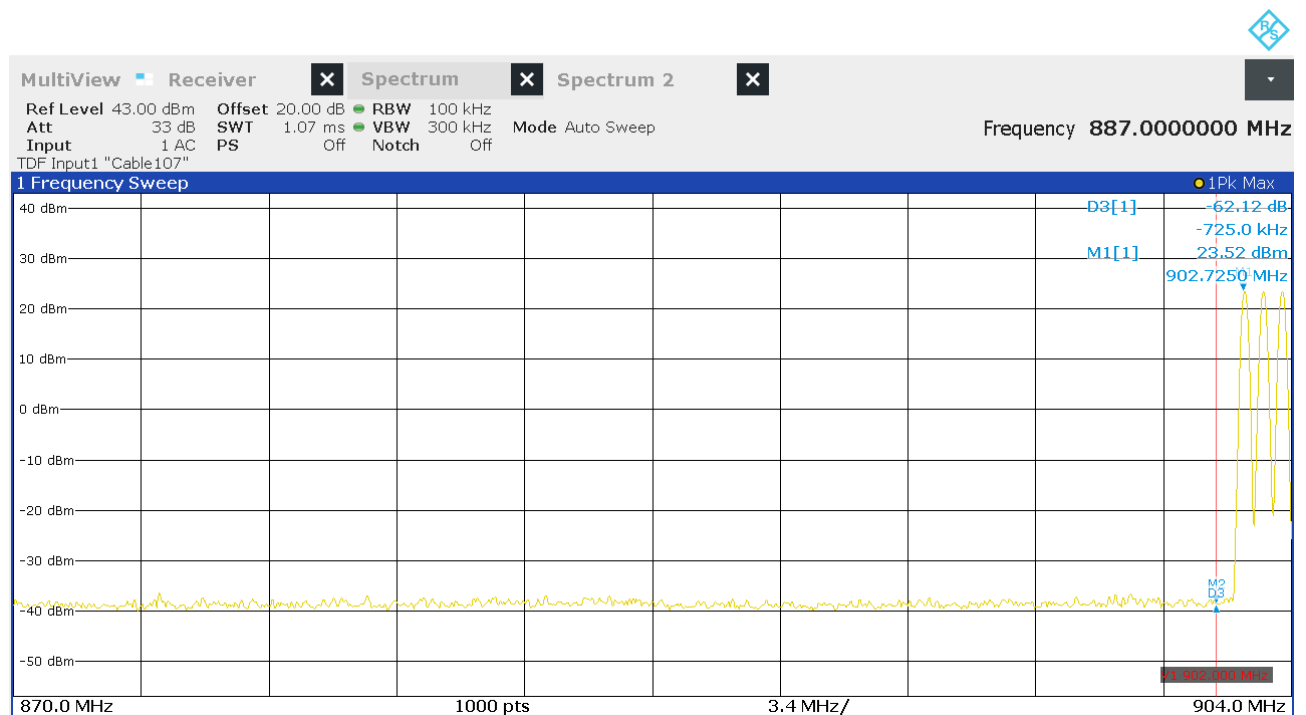
Figure 22: Chart of lower band-edge measurement in hopping mode
