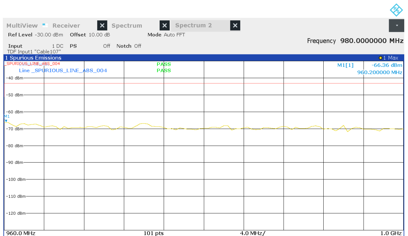
Figure 26: Chart of emissions test from 960 MHz to 1 GHz on lowest channel, Pk
