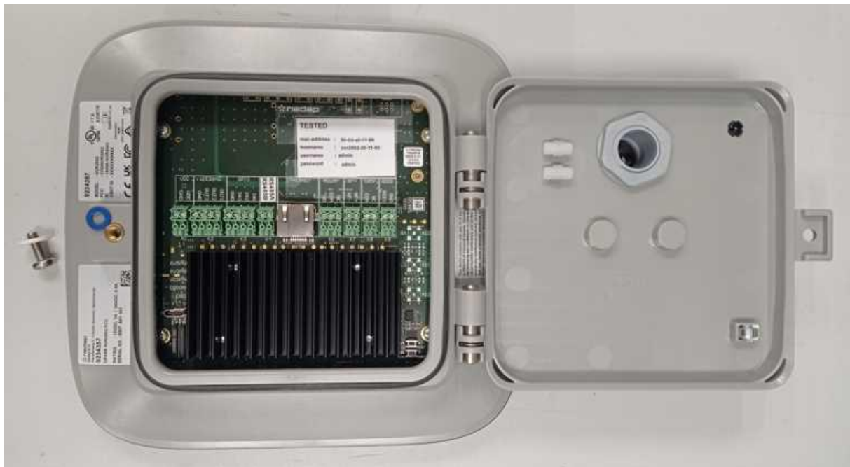
Fig.1 – Rear enclosure with access cover opened
