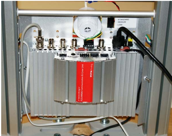
GSM/GPRS Module in the antenna FL-AS
