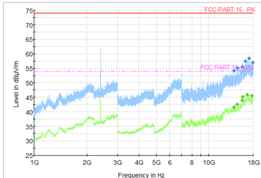
Fig. 52 Radiated Spurious Emission (8DPSK, Ch0, 1GHz ~ 18GHz)
