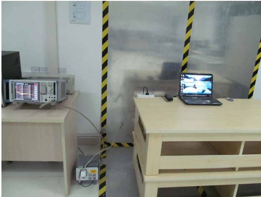
FCC LINE CONDUCTED EMISSION TEST SETUP
