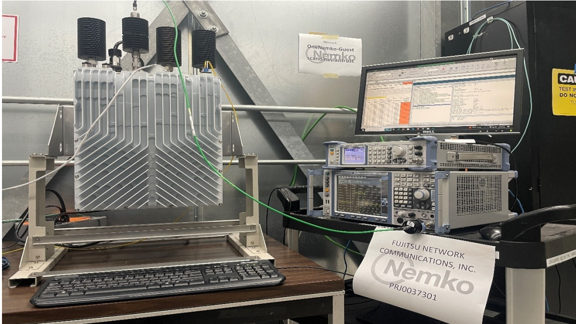
Figure 8 – Test setup (spectrum analyzer measurements)
