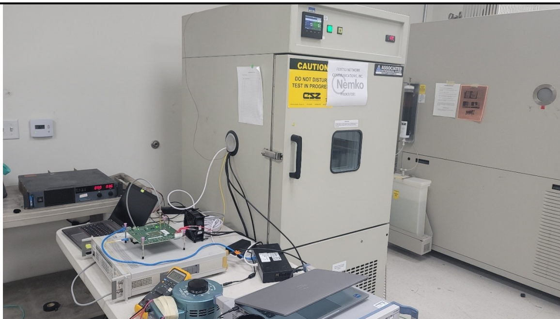
Figure 9 – Test setup (frequency stability test setup)
