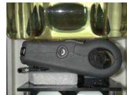
Figure 14.2 Hand SAR Test Setup
