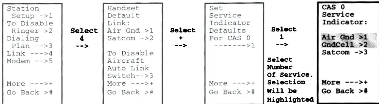
**MAGNASTAR C-2000 DIGITAL AIRBORNE TELEPHONE SYSTEM**
