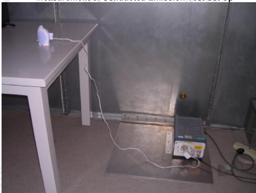
Measurement of Conducted Emission Test Set Up
