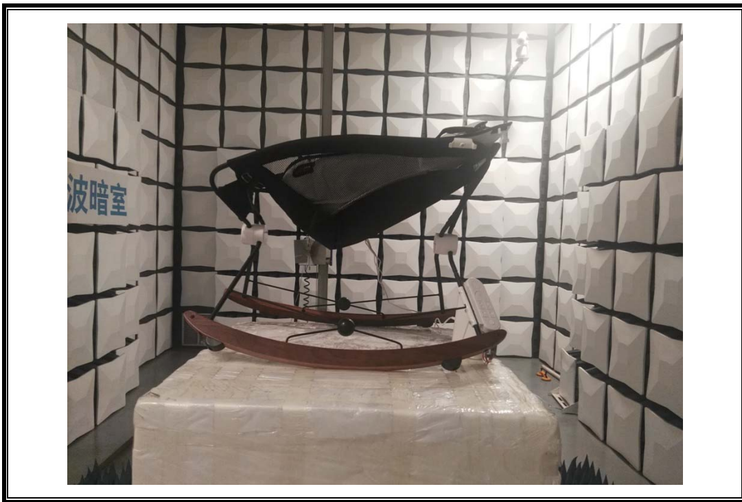
RADIATED RF MEASUREMENT SETUP (ABOVE 1 GHz)
