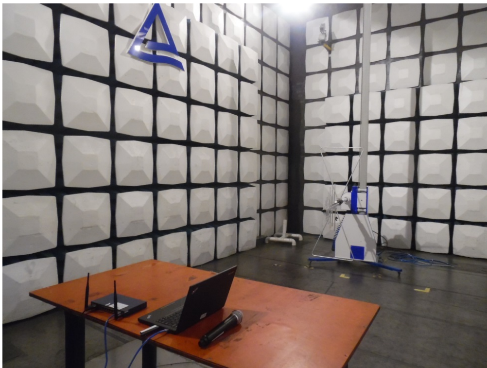
Photograph 2: Set-up for Radiated Emission (30MHz-6GHz)
