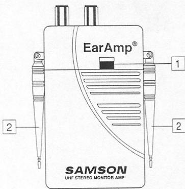
**1: Battery door release** - Press this latch gently upwards in order to open the battery door and access the controls contained within. When closing the battery door, swing it gently upwards until you hear this latch click.
