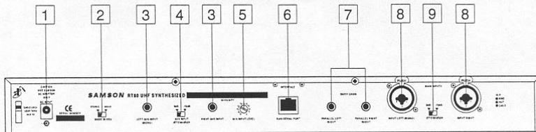
**1: DC input** - Connect the supplied power adapter here, using the strain relief as silkscreened on the rear panel. **WARNING:** The substitution of any other kind of power adapter can cause severe damage to the Wireless EarAmp® transmitter and will void your warranty.
