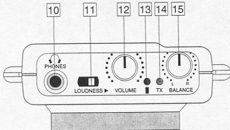
**10: Headphone jack** - Connect the supplied stereo earbuds (or third-party earpieces—see Appendix D on page 13 in this manual for more information) to this standard 1/8" (3.5 mm) mini-phone jack in order to monitor the signal being output by the Wireless EarAmp®. The level of the headphone signal is set by adjusting the Volume control (see #12 below). Maximum output is 200 mW @ 32 ohms.
