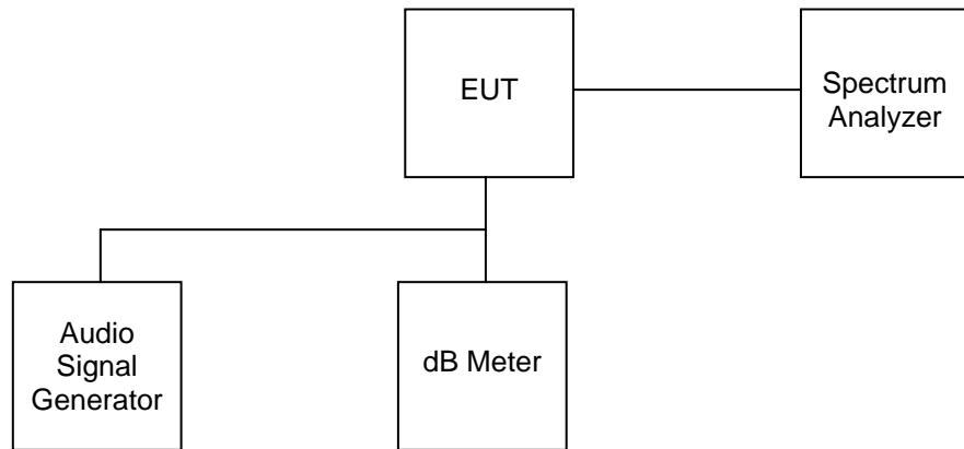
2. Other than single side band or independent sideband transmitters when modulated by a 2500Hz one at an input level 16dB greater than that necessary to produce 50 percent modulation. The input level shall be established at the frequency of maximum response of the audio modulation circuit.
