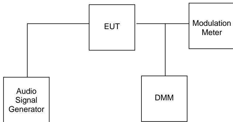
2. Apply a 1000Hz tone and adjust the audio frequency generator to produce 20% of the rated system deviation.
