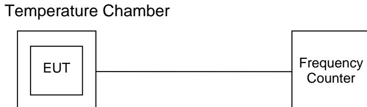
2. Set the Temperature Chamber to  $-30^{\circ}\text{C}$  and stabilize the EUT temperature for one hour. Turn the transmitter ON for two minutes.
