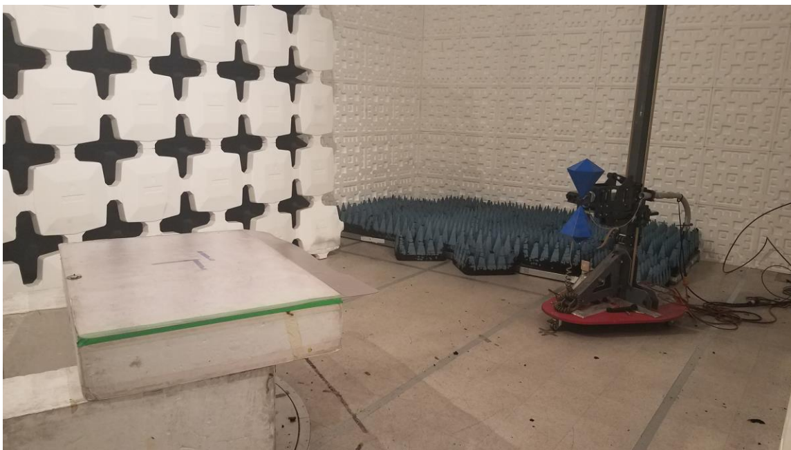
Figure 3. Radiated Emissions Test Setup, 30 MHz to 1000 MHz
