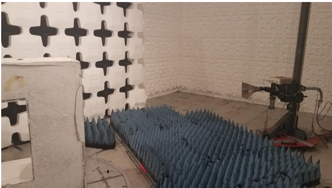
Figure 4. Radiated Emission Test Setup, above 1 GHz
