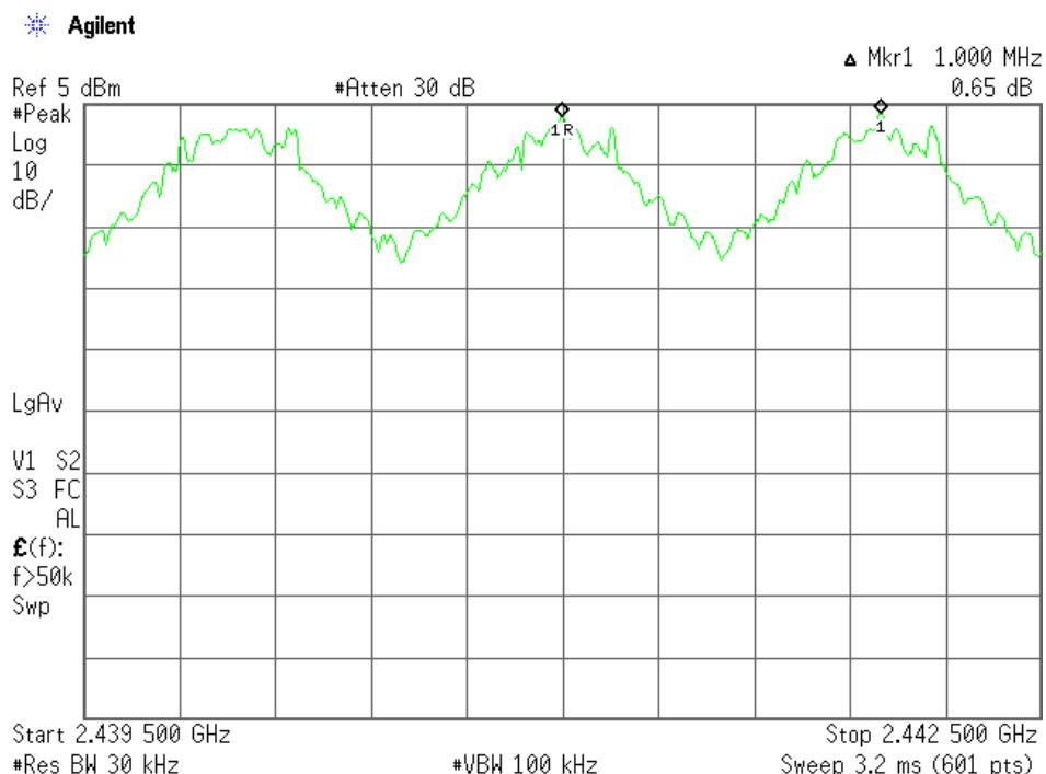
The hopping channel carrier frequencies are separated by a minimum of the 20 dB bandwidth of the hopping channel.
