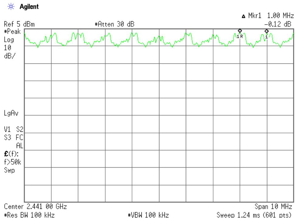
The hopping channel carrier frequencies are separated by a minimum of the two-thirds of the 20 dB bandwidth of the hopping channel.
