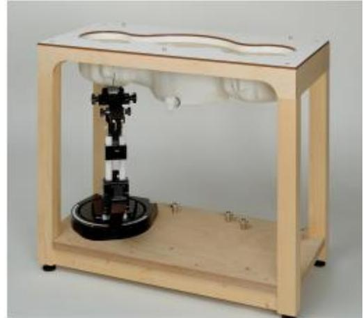
A white cover is provided to cover the phantom during off-periods to prevent water evaporation and changes in the liquid parameters. Free space scans of devices on top of this phantom cover are possible. Three reference marks are provided on the phantom counter. These reference marks are used to teach the absolute phantom position relative to the robot.
