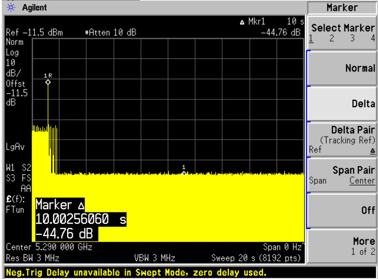
Type0 radar channel closing transmission time result:
