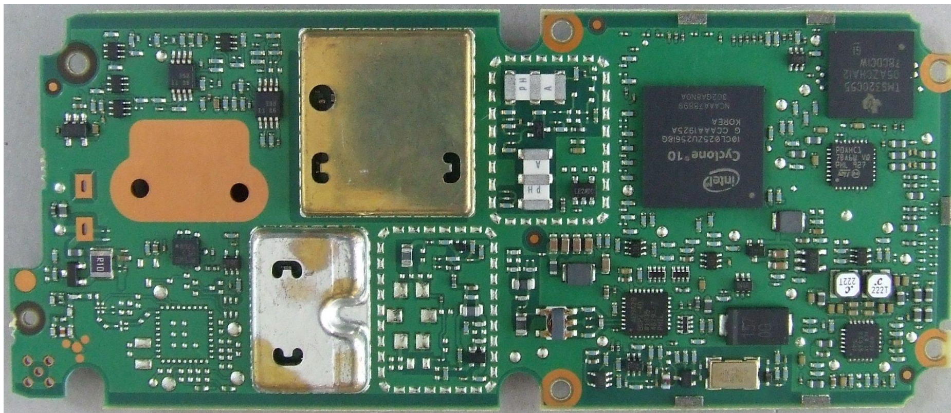
Photograph 03: Receive-Transmit PCB - bottom (with shields)
