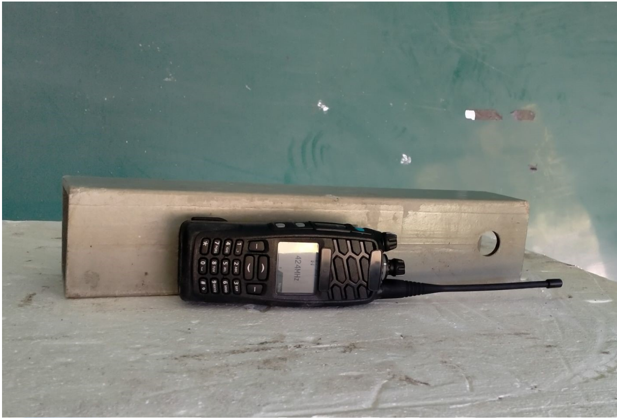
Test sample with UHF antenna attached: Z Plane – Laying on its Side
