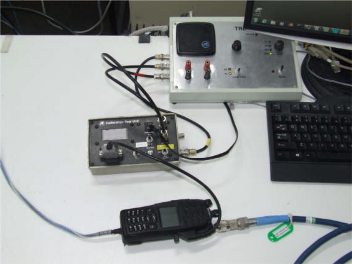
Photo showing the EUT connection to the test system using the customer supplied test box and battery eliminator.
